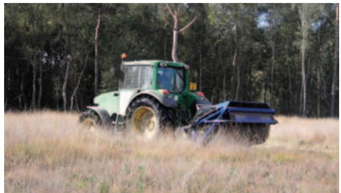
Cutting vegetation and collecting the cut material in one operation
